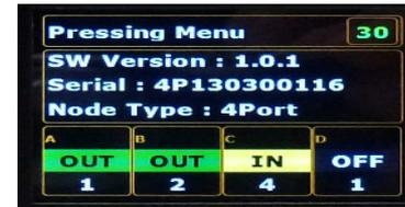
Identify Mode: identifies this MA 4Port Node by flashing the respective configuration line in the console/onPC (not implemented in version V2.8)
