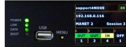
Hold button MENU as long until the desired menu appears. Release the button when in a menu adjustment is to be made. To change the setting, press the button briefly, the new setting is color-coded. After a short time display returns to the above menu.
